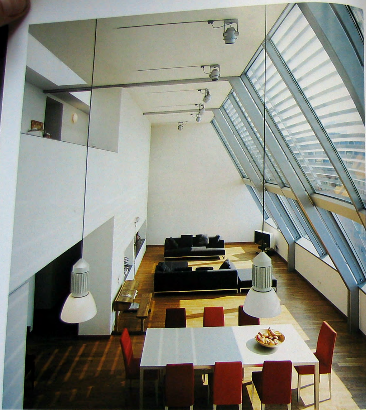
Aluminium, steel and glass dominate the 75-m 2 airy room, which is 5.50 m high at its highest point. The lights are from Bega and Erco. ■
