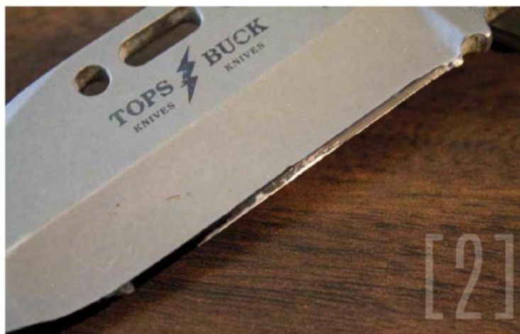
[2] The high wear on the marker indicates that this grind is too deep.
