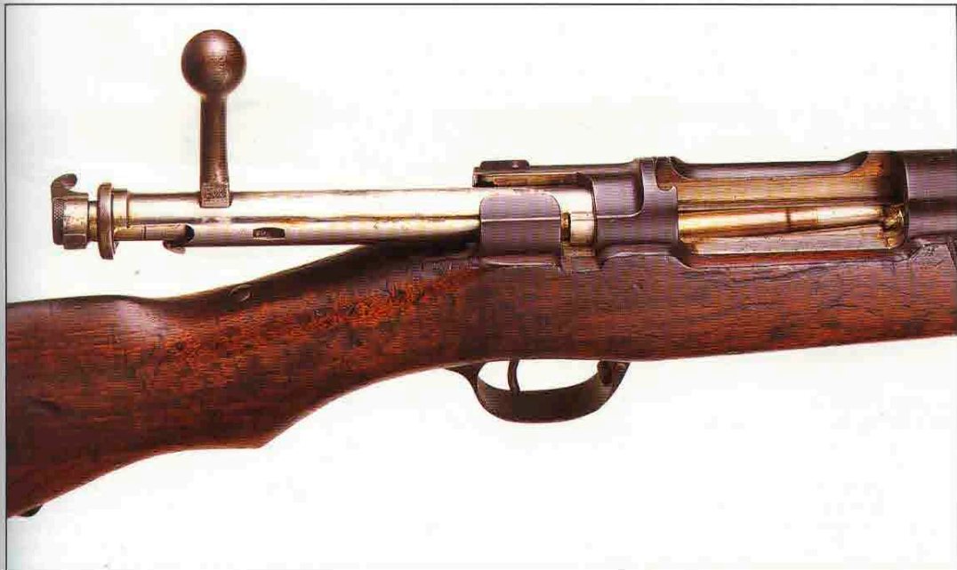
■ ABOVE: The Japanese Arisaka rifles were basically Mauser designs. This is the Meiji 30 Year type, introduced in 1897, chambered for the 6.5mm x 50 round and available as rifle and carbine.
