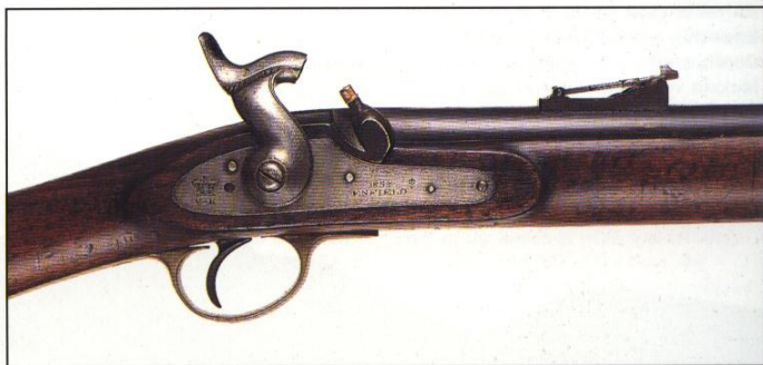
■ BELOW: This view of an Enfield 1853 Pattern rifle-musket shows very clearly how much simpler was the percussion cap than the flintlock system, with its cock, flint, frizzen, pan and touchhole.
