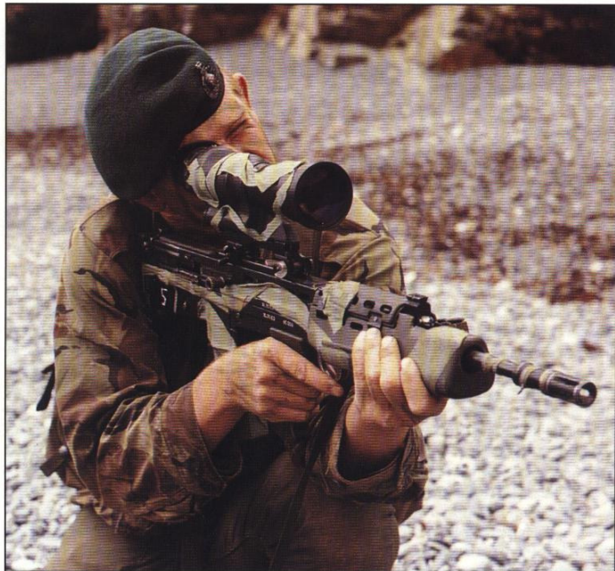
■ LEFT: This Royal Marine has used masking tape to break up the outline of his telescopically-sighted L85A1. The optional sight uses the same mount as the normal SUSAT unit.
