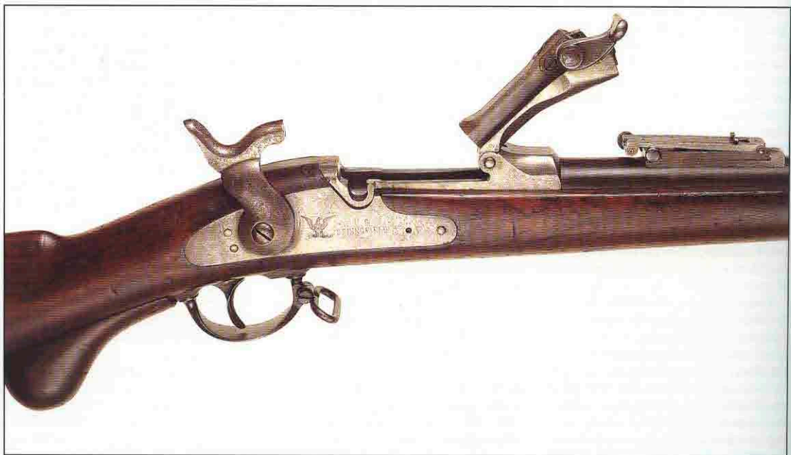
■ ABOVE: A beautifully preserved Allin-modified 'trapdoor' Springfield. These rifles were issued from the late 1860s and were not entirely superseded until well into the twentieth century.
