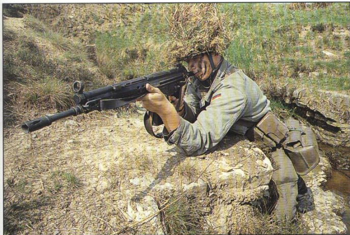
■ LEFT: A German infantryman with an extending-stock Heckler & Koch G3A4 rifle. The rifle was based on the Spanish CETME, which was itself developed from a Mauser design.
