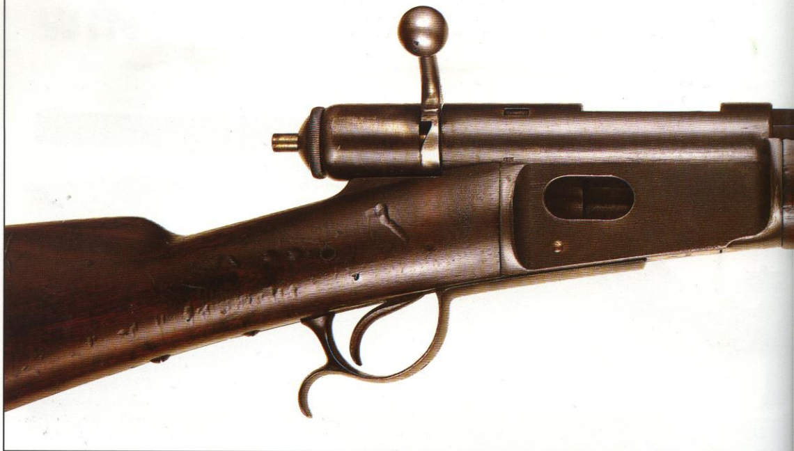
■ ABOVE: The Vetterli rifle in 10.4mm calibre was taken up by the Swiss Army in 1868. The first version was improved, and was superseded by the Model 1871, shown here.
