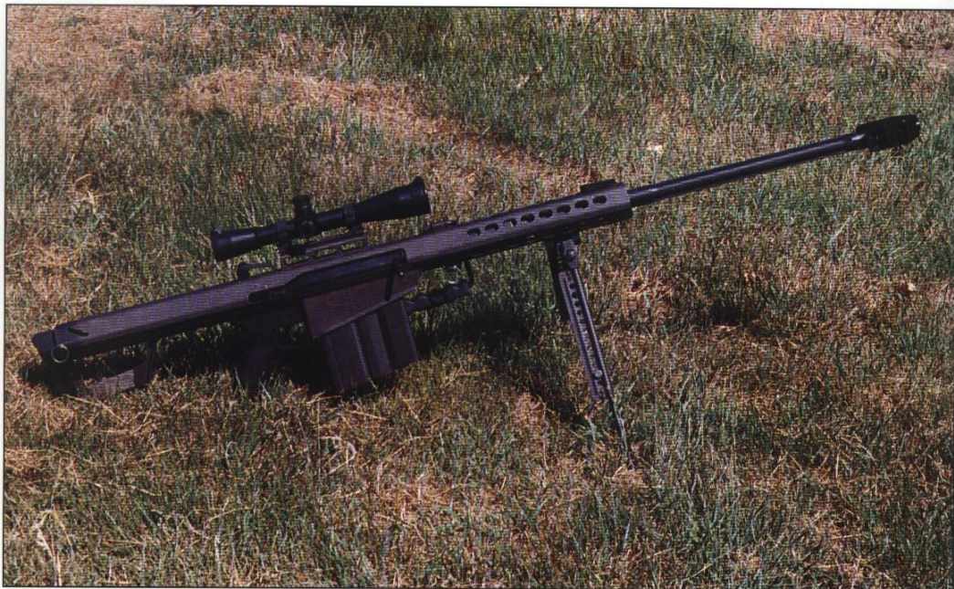
■ ABOVE: The Barrett Model 82 A-1 Light Fifty is one of the most powerful firearms on sale to the general public. It is chambered for the same .50in round as the Browning M2 machine gun.
