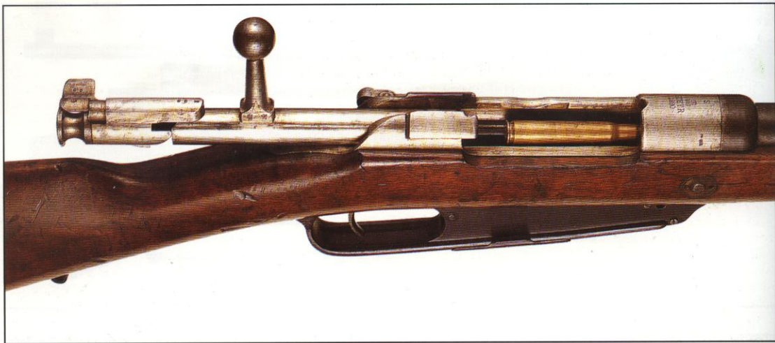
■ ABOVE: The German Infanteriegewehr 88 was poorly designed; the entire stock had to be re-barrelled (as this has been - note the 'S' incised into the breech case, indicating spitzer).
