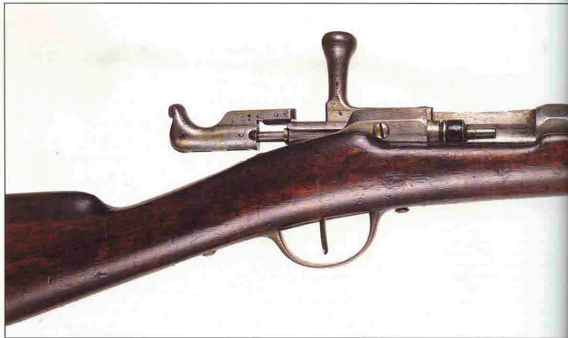
■ ABOVE: This photograph of an early model Chassepot (note the 1867 date of manufacture stamped into the barrel) shows clearly the shroud protecting the needle-like firing pin.
