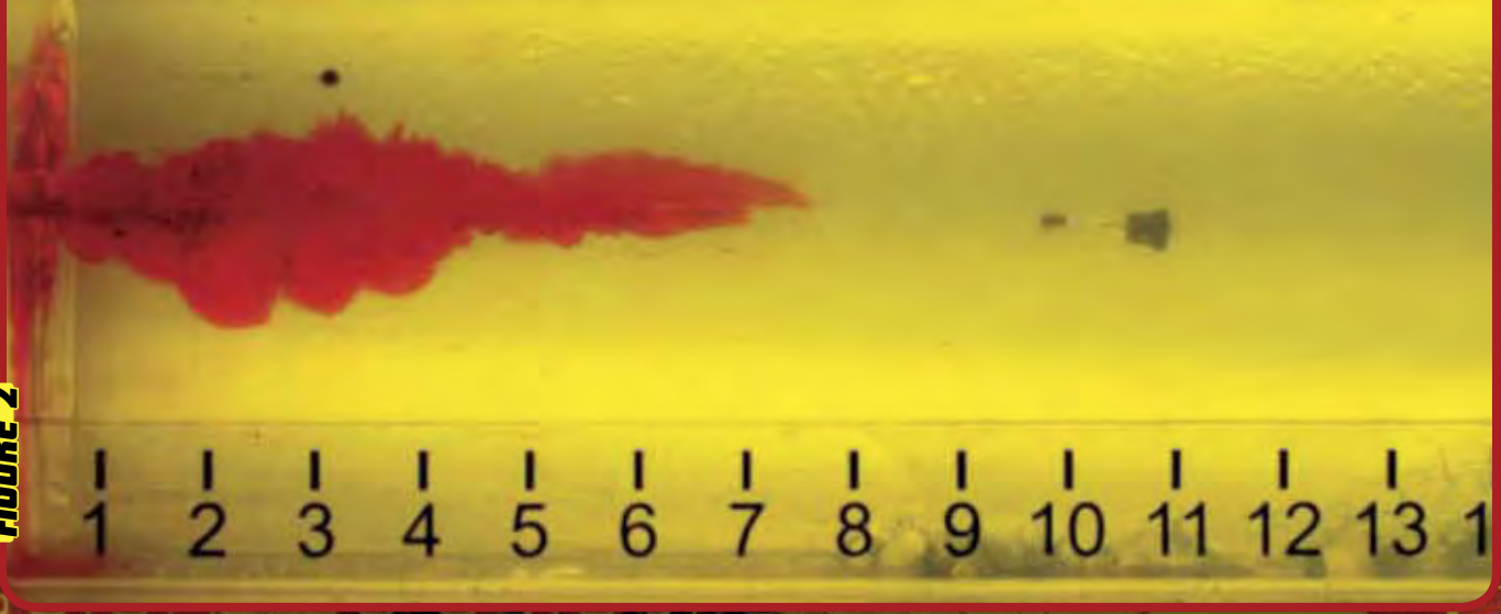
Heavy clothing penetration test in gel with the .32 NAA and 80-gr. FTX load.
