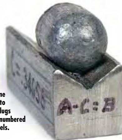
To begin slugging a barrel, you'll need something non-metallic to hammer with, and a pure lead slug significantly larger than the bore to be slugged. Duke likes to use round lead balls.
