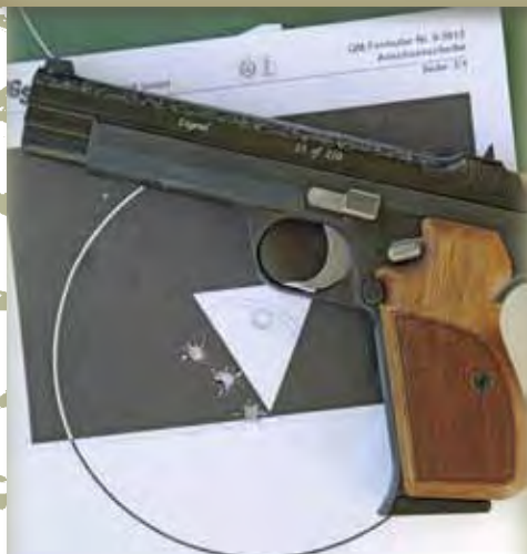
Traditionally, test targets were fired from 50 meters, with 2" being the accuracy standard. Recently SIG SAUER has been supplying 25-meter targets instead. This one measures 1.4".
