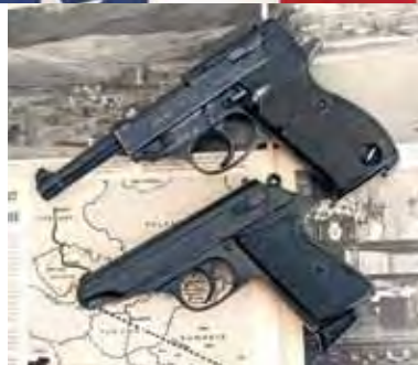
Walther P-38, PP: The first successful DA auto pistol was the Walther PP (bottom), a blowback design. The Walther P-38 (top) used the same concept on a locked-breech, service-size sidearm.
