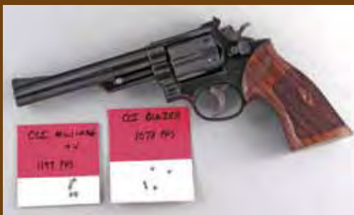
This S&W Model 53 (.22 Jet) is now usable once again thanks to the new .22 LR cylinder fabricated by Hamilton Bowen.
